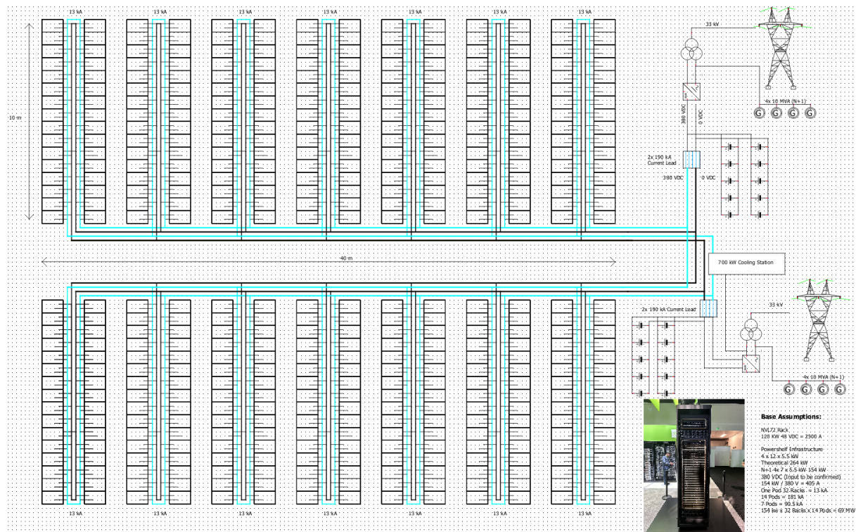
Figure 2 Electrical overview of the EOS data center. It includes two superconducting distribution lines, pod distribution, UPS, converters, transformers, grid connection and generators.
